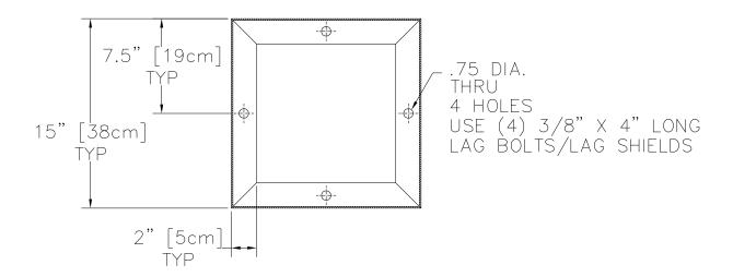
The AG812 is to be located on a **solid, non-combustible surface**, such as concrete. Mark the Gate location from the architect's drawings. Conduit for the Gate motor and controls must be brought to the stub-up area within the Gate's bottom opening (shown above). Foundation bolt location can be marked from the Gate itself or from a template (Delta P/N D03180).
